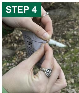
Remove the clear cap from the conductivity sensor and rinse the now exposed probe with distilled water. Always rinse your meter 3 times before taking a new conductivity measurement. Dry it with a clean tissue.
